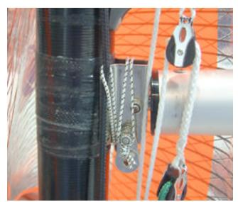
You can use your existing halyard but we suggest you rig it as follows. After the main is fully hoisted, flick the fall of the halyard into the open hook pictured below at the top of the lower section, hold the halyard close to the gooseneck and push a
