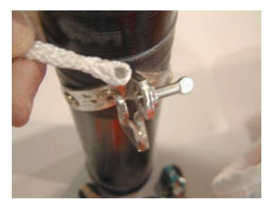
The pictures show the recommended cunningham arrangement. A loose spectra braid has been used which is easily spliced even by an amateur. A loop has been created in the middle of the line and this is hooked over the pin of the twist shackle that holds the vang.
