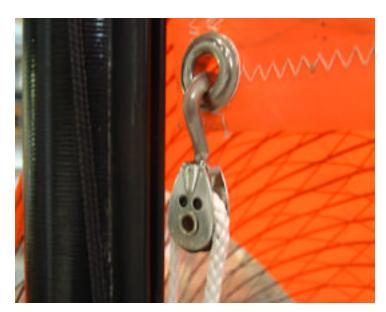
The existing system of a rope passing through the grommet and terminating in a block can still be used but the system shown, using a hook block is simpler and allows easier de-rigging as the whole system can stay with the mast.
