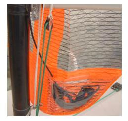
The halyard is shown secured on the starboard side of the spar in these pictures for ease of illustration. It should be passed through the open hook at the top of the lower mast then brought down and tied off as shown **but on the port side of the mast** since the pocket is on that side. Now stow the tail, as shown in the picture, in the pocket at the bottom of the cuff.
