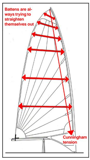
open itself up. The only way to de-power is to let the boom down to leeward but there will still be virtually no twist in the leech. This lack of twist makes it very hard for a lighter person in heavy air and it is the same problem that exists with the Laser, the Radial and the Europe.
