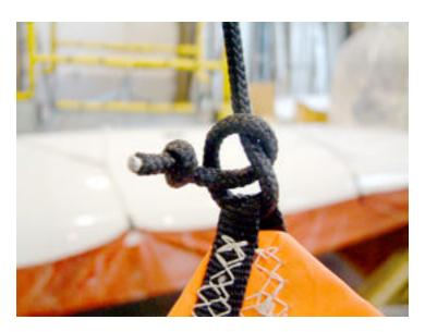
The sail needs to be hoisted very near to the sheave so do not tie a long bowline in the halyard. Do a single overhand knot then follow with another overhand as shown. The final sail has a
