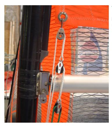
This shows the complete 8:1 system in place. Note that the tack of the sail is well up above the boom for light air. In heavy air, it will be down very near, or at, boom level.
